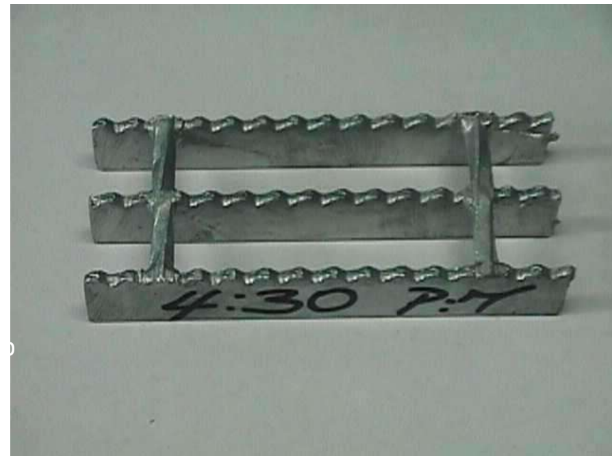
Figure 12. (a) Part of "grating" fluxed with Galvacid® flux HSC-PF Free of Ammonium and subsequently submitted to the environment by two hours before Galvanizing. Rejections not observed in the final galvanization. (b) Piece of "Grating" fluxed with Galvacid® Flux HSC-PF Ammonium Free and subsequently exposed to the environment for 4 hours before its galvanizing. Rejections not observed in the final galvanization.
