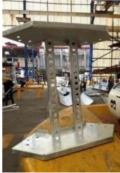
Figure 8. (a) Electrical steel article with complex geometry, fluxed with the new Galvacid® Flux HSC-PF Ammonium Free. It can be seen that the surface has turned black, typical of the “High Surface Conversion”, unique characteristic of this new development. (b) The same part already galvanized, showing perfect galvanization, gloss, free of bare dots zinc coating. Discontinuous Process (Batch) Immermek, Mexico 2019.
