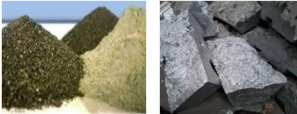
Figure 6. On the left, ashes of Zinc, on the right "dross". Examples of waste of zinc during the process of galvanizing. The use of this new technology has proven that these byproducts can be significantly reduced, which implies considerable saving of zinc for the galvanizer.
