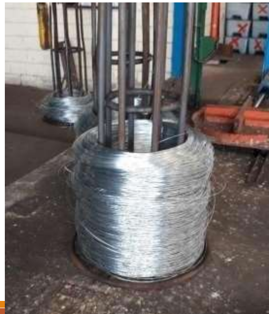
Figure 7. Continuous wire process. Finished galvanized wire, with 100% ammonium removal. A galvanized with good brightness and without rejections is observed. Wires Yaracuy – Venezuela. February 2017
