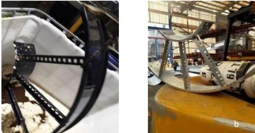
Figure 11. (a) Piece of tower of electricity with complex geometry, fluxed with the new Galvacid® flux HSC-PF Free of Ammonium. It can be observed that the surface is turned black, typical of the “High Surface Conversion”, unique characteristic of this new development. (b) The same part already galvanized, with a perfect galvanization.
