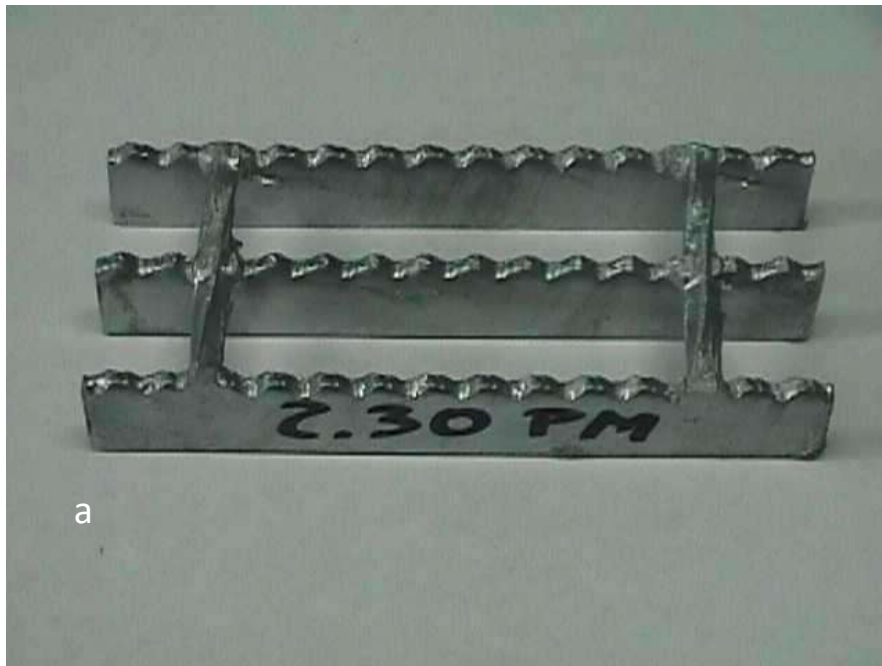
Figure 12. (a) Part of "grating" fluxed with Galvacid® flux HSC-PF Free of Ammonium and subsequently submitted to the environment by two hours before Galvanizing. Rejections not observed in the final galvanization. (b) Piece of "Grating" fluxed with Galvacid® Flux HSC-PF Ammonium Free and subsequently exposed to the environment for 4 hours before its galvanizing. Rejections not observed in the final galvanization.
