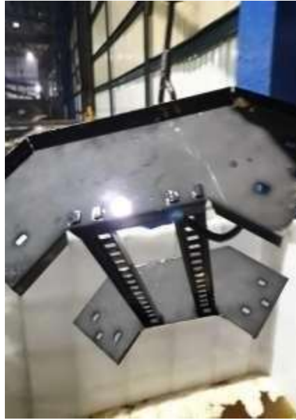
Figure 8. (a) Electrical steel article with complex geometry, fluxed with the new Galvacid® Flux HSC-PF Ammonium Free. It can be seen that the surface has turned black, typical of the “High Surface Conversion”, unique characteristic of this new development. (b) The same part already galvanized, showing perfect galvanization, gloss, free of bare dots zinc coating. Discontinuous Process (Batch) Immermek, Mexico 2019.
